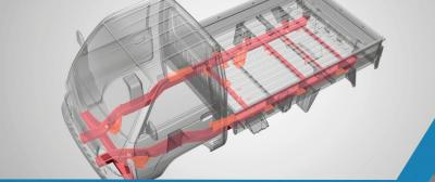
Strong chassis frame made from rust resistant steel.
