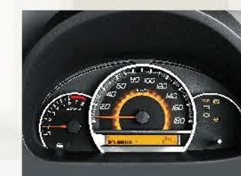
Digital fuel indicator with double trip meter
