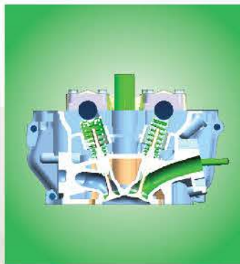
Special material Valve Seats for better durability
