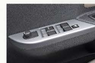
Electric ORVM & power-window controls on driver's arm-rest
